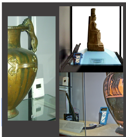
Indagini microclimatiche in teche espositive
